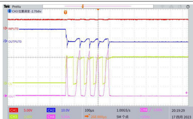
Figure9.3 Over current protection in retry mode
